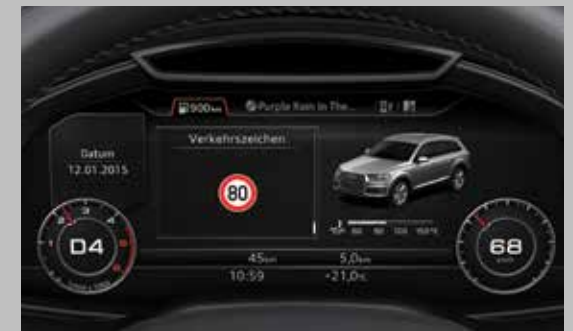
Image shows Audi Virtual Cockpit in infotainment view with optional Traffic sign recognition (available as part of the Dynamic Pack)
